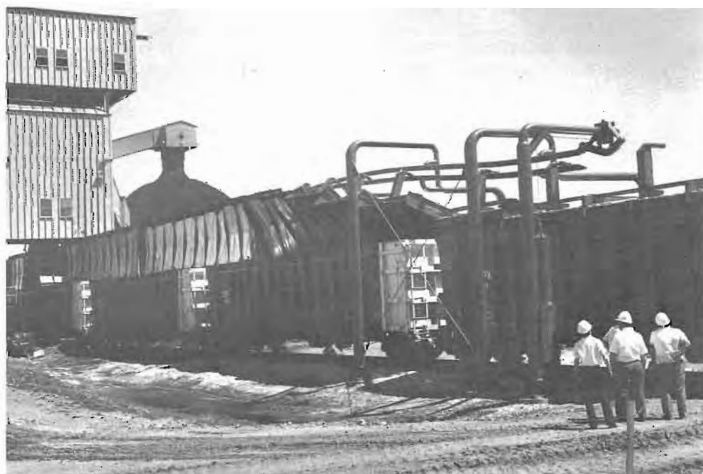
Milwaukee Road technicians observe scroll mechanism as it lowers hinged lids over loaded gondola cars.
