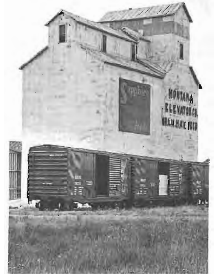
Box cars with paper grain doors installed await loading at grain elevator near Lewistown, Mont.
