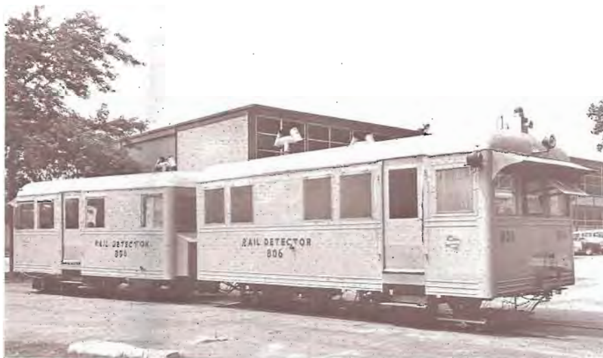
Rail detector car No. 806 rests on a test track outside of the AAR Technical Center in Chicago where the new equipment was adapted to the existing test car. Test equipment is suspended beneath the right half of the car. The left half is the front end and contains the engine that drives the car.
