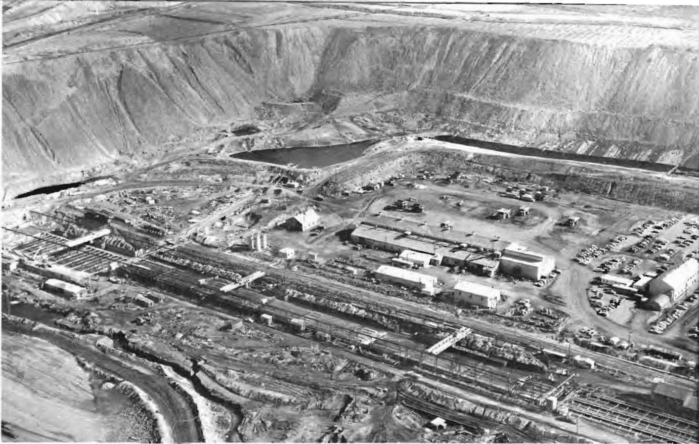
An aerial view of Anaconda Company's precipitation plant in Butte, Mont. Leach dumps are shown in the upper half of the picture. Anaconda Company photo.
