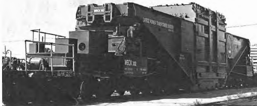
A 500 ton transformer, built by the Westinghouse Corporation and destined for Public Power in Elkhorn, Neb., is shown as it awaited departure from Savanna (Ill.) Yard on Aug. 29. The transformer, valued at over $600,000, was handled by the Milwaukee Road from Savanna to Council Bluffs, Iowa. (Photo by R. Milton Clark, Savanna, Ill.)
