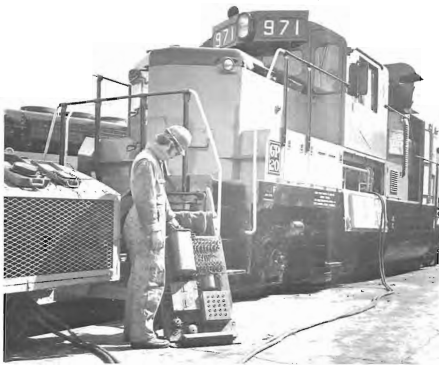
Electrician Ted Veres (foreground) and Machinist Ernest Hirshman are shown performing a load test on unit 971 at the Milwaukee Shops. Each unit undergoes a thorough load test in the shop and receives a comprehensive road test before it is released into train service.
