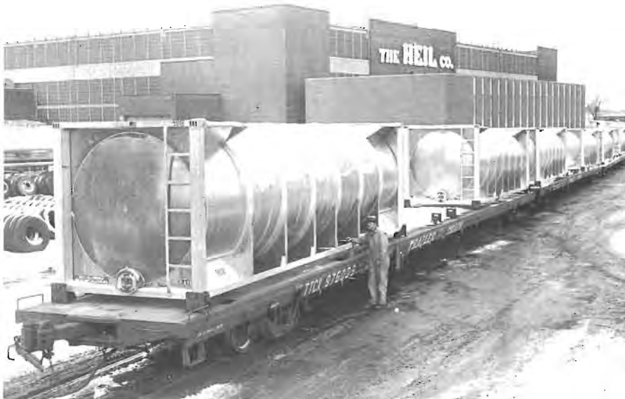
325 ALUMINUM CONTAINERS manufactured by the Heil Company of Milwaukee recently began movement over the Milwaukee Road on their way to Perth Amboy, N. J. The containers, each with a 1,324 cubic foot capacity, are designed for the transportation of prilled pellets (approximately 1/16 inch balls) of petroleum-based plastic between Puerto Rico and Perth Amboy. The total shipment will require 163 TTCX container cars, with two units loaded on each car.
