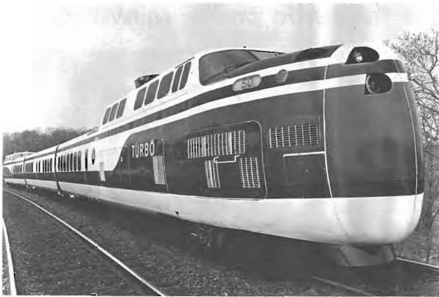
A three-car version of the TurboTrains currently in service between New York and Boston as part of the Department of Transportation's Northeast Corridor high speed ground transportation demonstration project. Bidirectional capability eliminates turn-around time at terminals.
