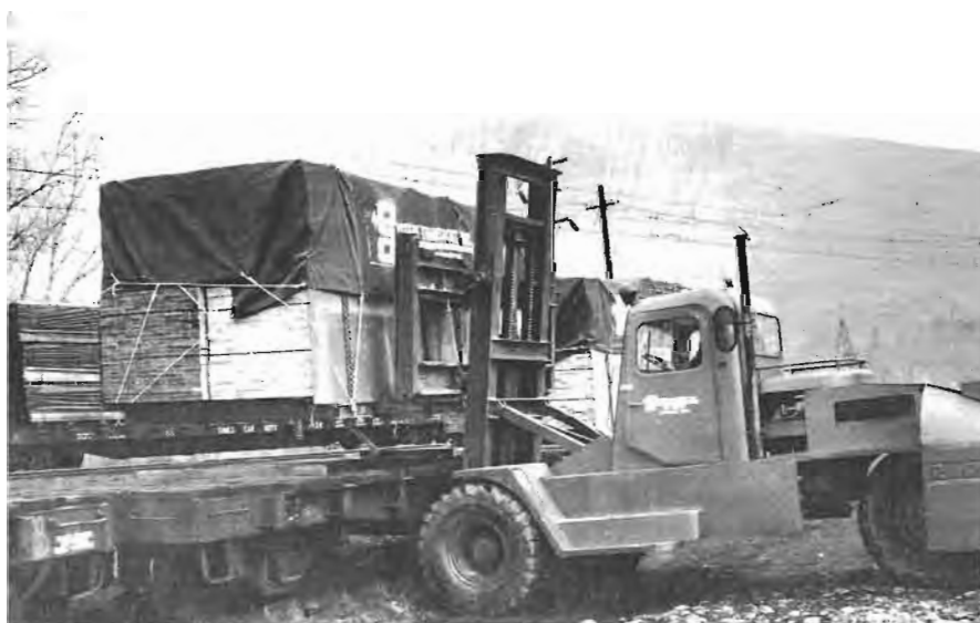
A "container flat" is loaded onto a railroad flatcar by a fork lift truck. Each container will hold about 20,000 pounds of dressed lumber.
