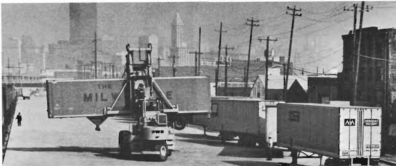
The Piggy Packer shows its muscle. It has a lifting capacity of 70,000 pounds and can transfer a container or piggyback
