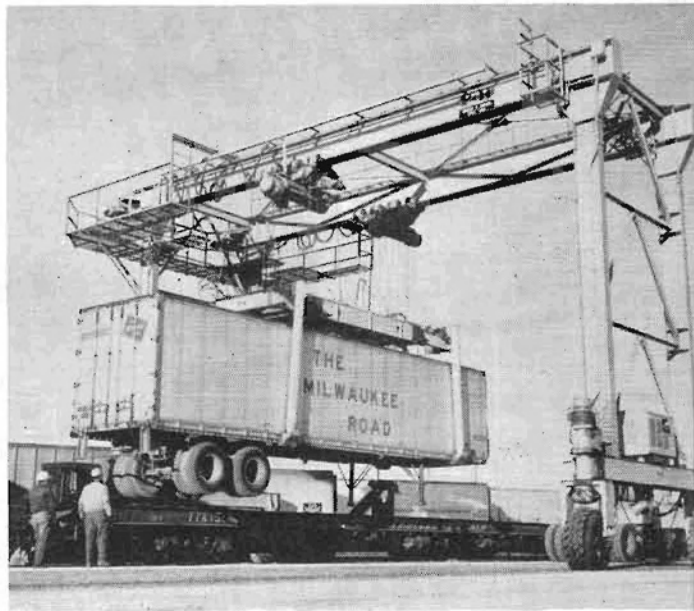
A close-up of the straddle crane, the work horse for most of the loading and unloading of trailer vans at Piggyback Park, placing a van on a flatcar.
