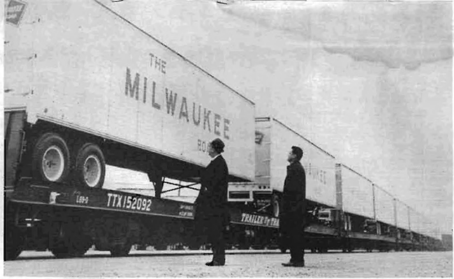
The first of the 250 new 40-foot piggyback trailers acquired by the road in 1965 are examined by P. L. Cowling, vice president and general manager of the Milwaukee Motor Transportation Company (left), and C. E. Goldsmith, manager of MMTC eastern operations. Two hundred are heavy duty refrigerator units equipped with meat rails, although they are designed for handling other commodities requiring refrigeration, and the other 50 are "dry van" units. Built to MMTC specifications, the refrigerated vans have fiberglass linings, and the dry van interiors are lined with a special epoxy paint which is easily cleaned and is non-toxic to perishables.
