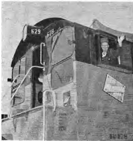
At work in the Everett, Wash., yard, Engineer Lawrence Griffin waves from the cab of a 1,200 horsepower diesel-electric switch engine.
