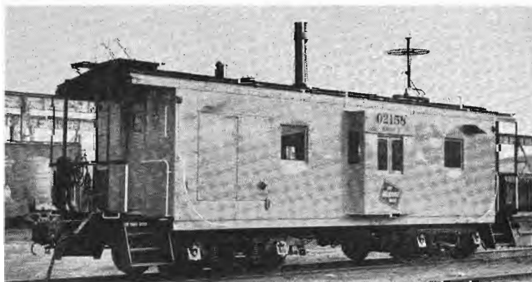
The "new look" in cabooses, with the number above the bay for easier identification and the trademark below.
