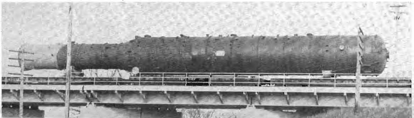
LONGEST AND WIDEST LOAD ever handled by the Milwaukee Road was this oil tank, 120 feet long and 14 feet in diameter, shipped recently on three flat cars from Eagle Ford, Tex., to the Great Northern Oil Company at Roseport, Minn., which the Milwaukee moved from Kansas City to its Austin, Minn., junction with the Chicago Great Western. The Milwaukee has handled longer and wider loads, but in combined dimensions this was the record.
