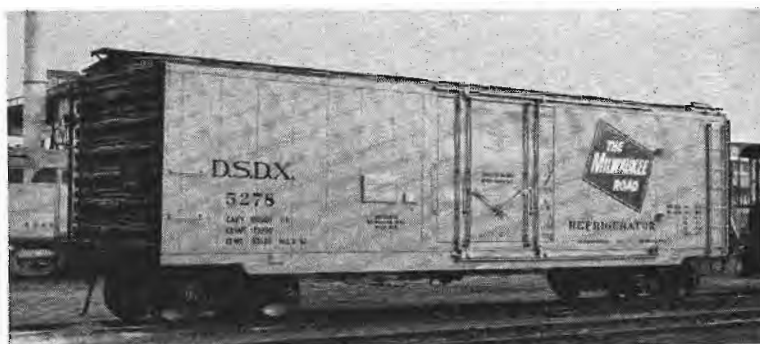
Modernized look of the rebuilt refrigerator cars, showing the 8-foot plug replacement for the old style four-foot door.
