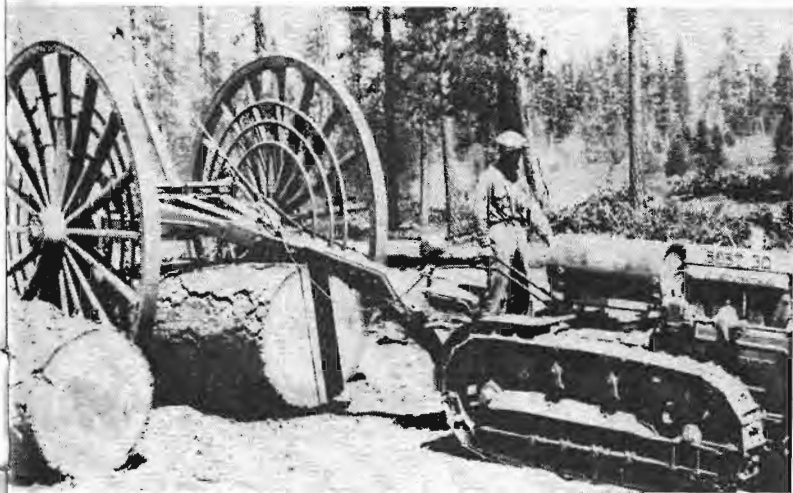
Gasoline powered tractors replace horses for hauling logs to the railroad. Pictured is an early model tractor and a high wheeled logging arch used in the operation.
