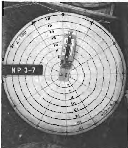
Laboratory shot of a roll of newsprint with an impact recorder attached to the top, undergoing shock in an incline contour test at the Association of American Railroads research center in Chicago. The numbers on the roll indicate where impact starts. The out-of-round condition at the right is known as "starring".
