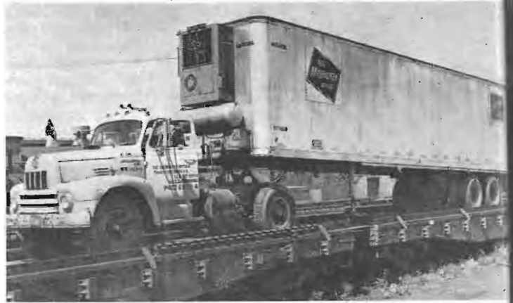
NEW T.O.F.C. FLEET presently being acquired by the Milwaukee includes 60 of these 39-foot Flexi-Van "Lamicoolers" equipped with Thermo-King freezing units, plus 40 vans of the 40-foot insulated type. The Thermo-King freezer, a heavy duty propane fueled unit featuring an automatic (heat-cool) switch, is capable of maintaining a temperature of zero or lower. In this picture taken at the TOFC terminal at Bensenville Yard, Milwaukee Motor Transportation Company Driver Leonard Kucharski is preparing to remove it from the flat car.
