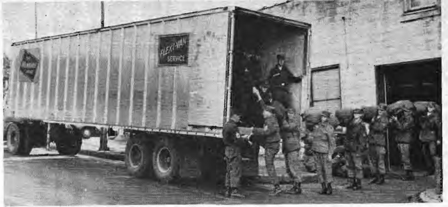
National Guardsmen in training at the Eau Claire, Wis., Armory place their personal baggage aboard a Flexi-Van for hauling by highway to La Crosse, Wis., where the van was loaded onto a Flexi-Van flat car.
