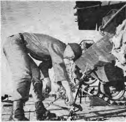
A member of an armor unit tightens a tie-down cable on a tank loaded aboard a flat car at Camp McCoy, Wis.
