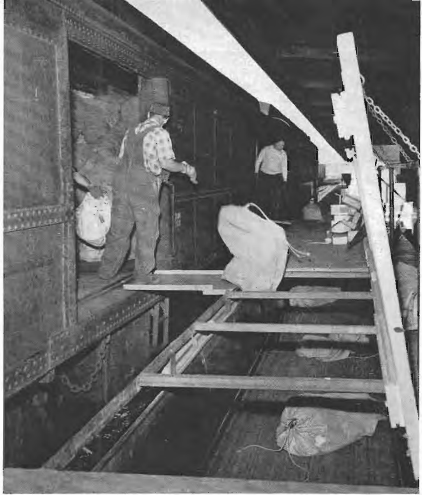
Mail sacks and pouches being unloaded onto a conveyor belt which carries them from the train platform to the sorting floor in the basement of the St. Paul Union Depot. St. Paul is the central working point for a large percentage of mail originating and terminating in Wisconsin, Iowa, Minnesota and North and South Dakota. Most of it moves by rail.
