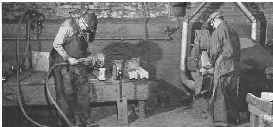
In the chipping room at the Milwaukee shops foundry, goggles go on at the door. Shown here grinding steel castings are Mike Tedich (left) and Paul Zaremba.
