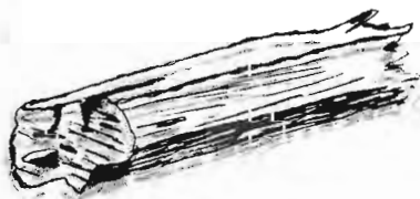
This untreated red oak tie failed after five years service
