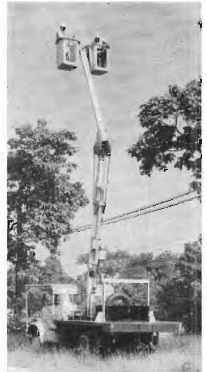
Nothing up there to trim, but the Skyworker demonstrates that, when necessary, it can reach 40 feet straight up. The baskets are kept in an upright position at all times.
