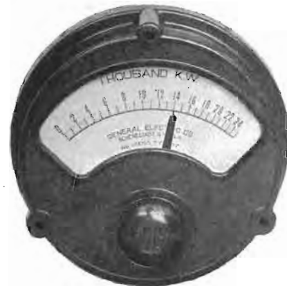
Fig. 4. Indicating Kilowatt Totalizer. Dispatcher's Office
