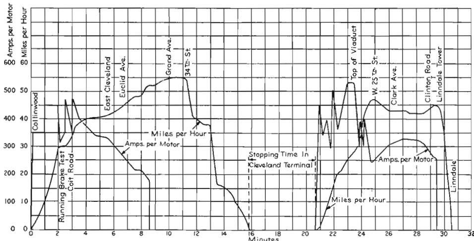
FIG. 4—SPEED-CURRENT-TIME CURVES FOR "THE 20TH CENTURY LIMITED" FROM COLLINWOOD TO LINNDALE, DEC. 2, 1931. TRAILING TONS, 1,100. CLEVELAND UNION TERMINALS ELECTRIFICATION
