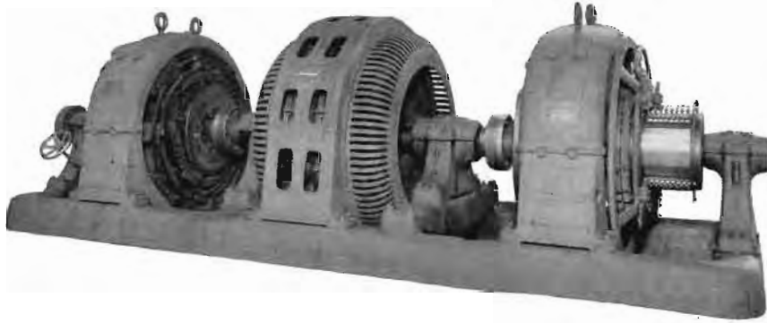
THREE UNIT 1000 KW., 2400-VOLT D-C. MOTOR-GENERATOR SET
