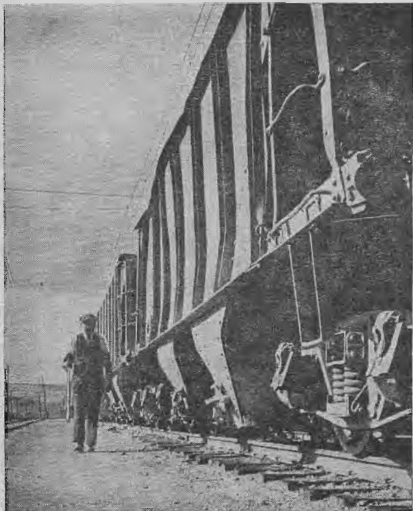
REAR BRAKEMAN walks along train, inspecting the air couplings and journal boxes. Locale is West Butte yard, where the Anaconda-bound train picks up initial tonnage, later filling out the train at Rocker
