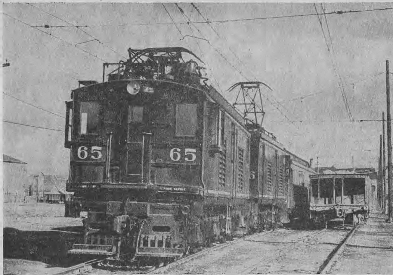
TWO-UNIT electric puts passenger car on the rear end of string of empties bound for Butte. Engine will couple coach on, then other end of the train
