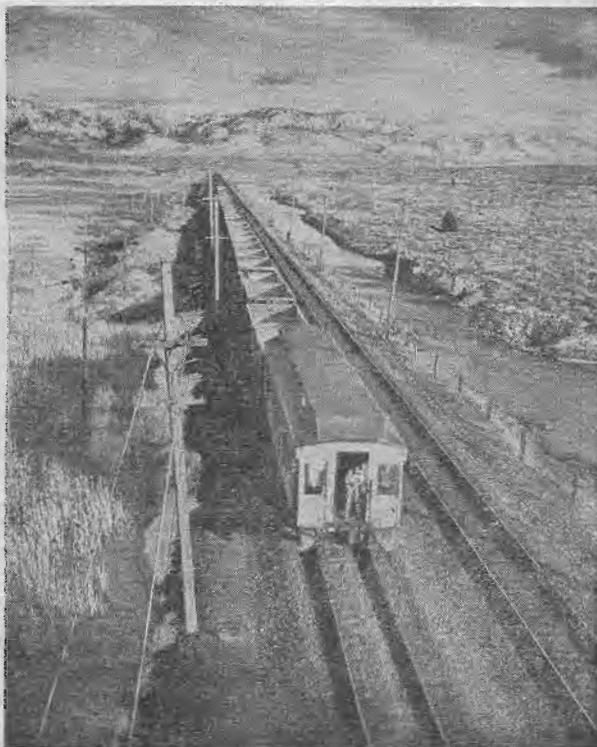
TWO UNITS start a string of loaded dumps for the twisting line that goes up the hill to the smelter from East Anaconda yard
