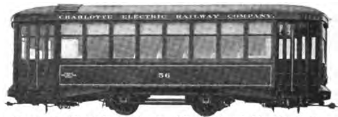
Charlotte Electric Railway—Single-Truck Vestibule Car
