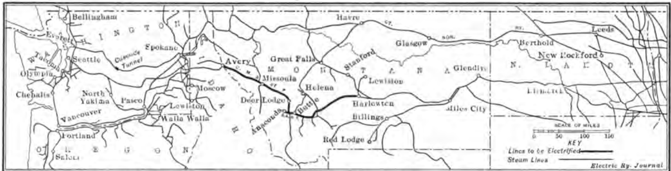
American Electrifications—Map of Electrified Lines in the Northwest, Showing Route of Chicago, Milwaukee & Puget Sound Railway
