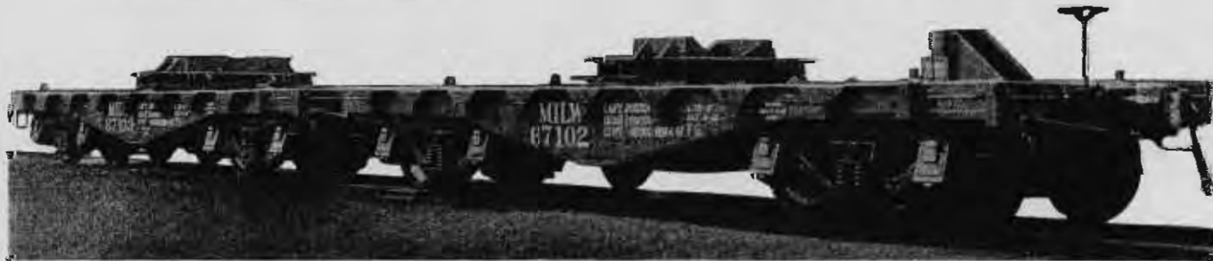
Specially designed, 100-ton capacity steel flat cars, used in pairs for the transportation of large naval guns
